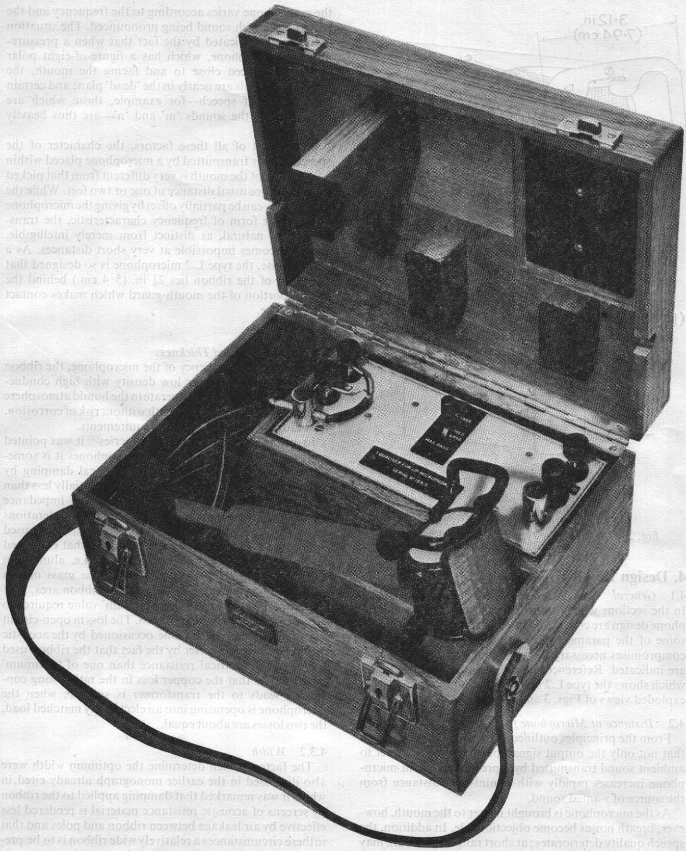
Fig. 1.— Microphone type L.2 with carrying case and variable equalizer
