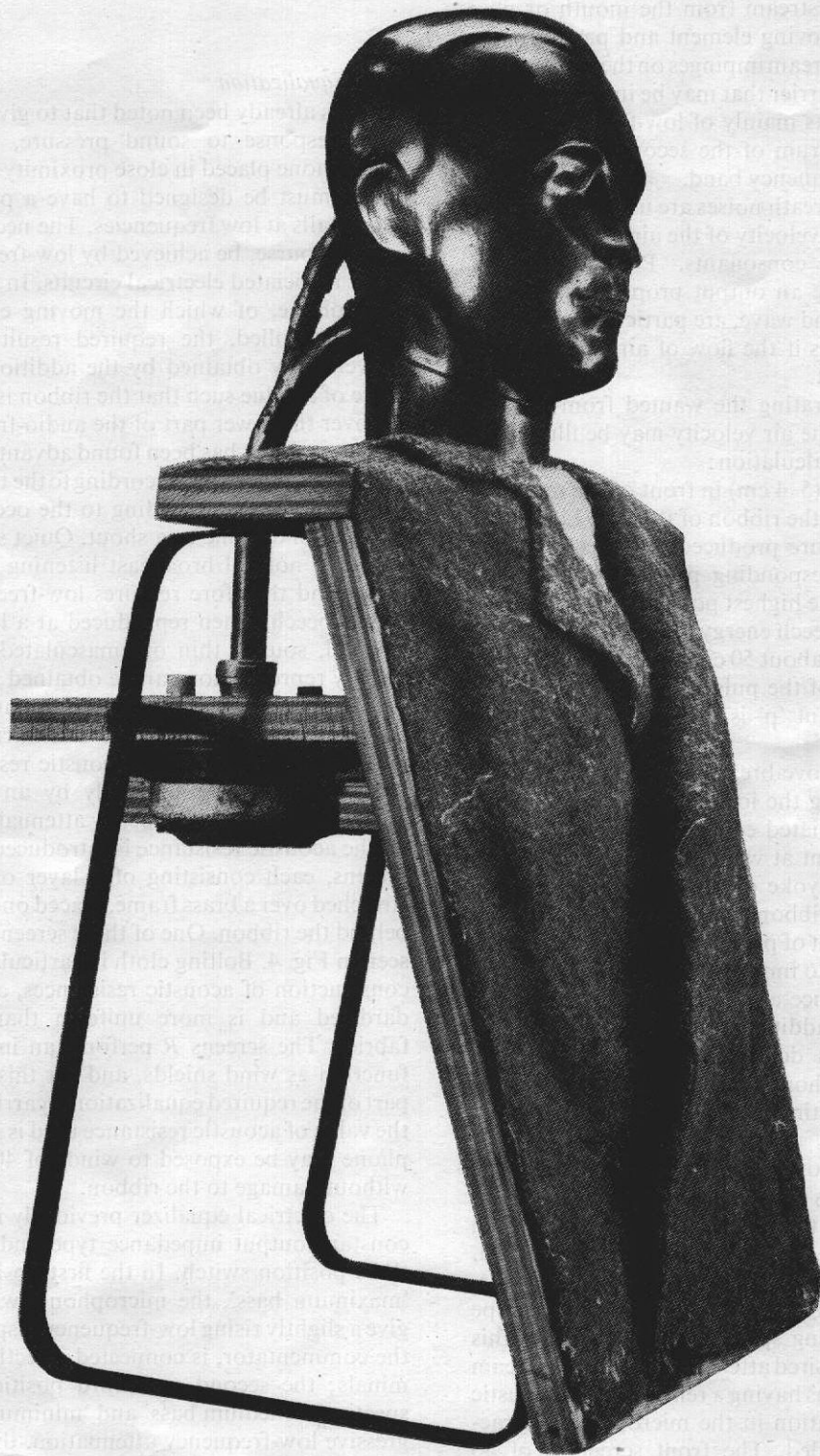
Fig. 5 — Artificial head used to measure the response of lip microphones
